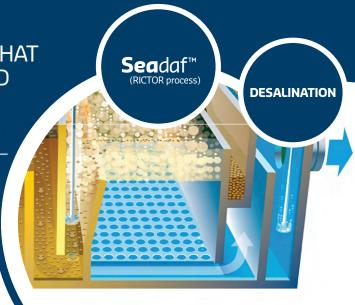
Seadaf™ is an air flotation system for clarifying seawater. Its unique design allows the treatment of very large volumes of water.
